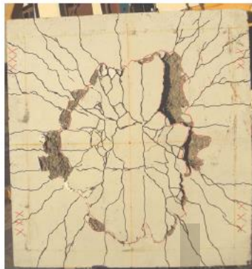
Fig. 8 Cracking pattern on tension surface at ultimate load for slab XXX and CF0 from experimental results.
